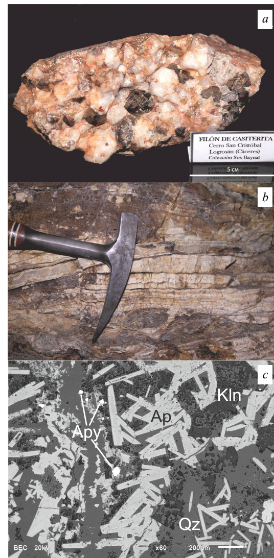
Fig.2. External appearance of the rocks under investigation: a – quartz-cassiterite druse from greisens, museum exhibit from Logrosán village; b – quartz-apatite vein, under exposure and through electronic microscope; c – image from back-scattered electrons
